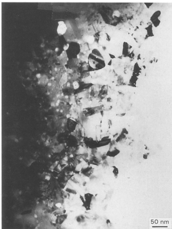
Figure 6 TEM micrograph of LG Ni deposit (Consort III) with sulfamate electrolyte and Au substrate.
